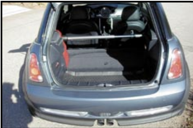
With the back seats out and the sound proofing removed, the MINI Cooper loses 200 pounds. Photo by Dave Stall
