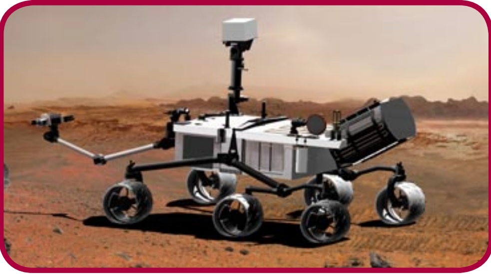
The full-sized prototype Mars Rover, as large as a small SUV. With its robotic arm extended forward, the rover is almost 15 feet long! Rover has six wheels, a tall mast (with the robot's "eyes") and numerous scientific instruments. The Mars Rover is on display at the Reuben Science Center. Photo courtesy of Reuben H. Fleet Science Center
